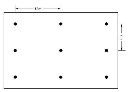
Spacing layout to achieve 160 lux maintained average (as per AS/NZS 1680) in an open warehouse with installation height of 12m.
