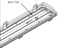
Fit the gear tray to the base and lock in position with the quarter turn fasteners. Installation positions to maintain IP rating
