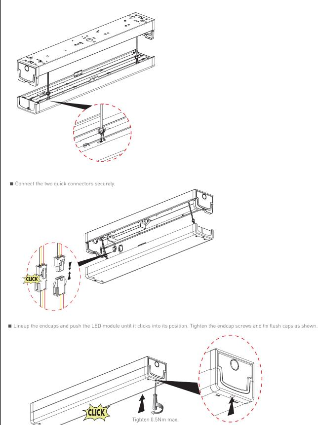
Fit flush cap on screw hole
