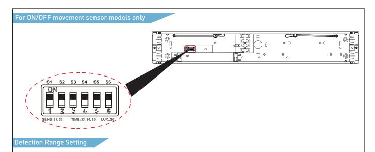
When installed at a height of 2.5m, the minimum setting will give a circular detection range of 2m radius and a maximum detection range of 10m radius. Switch position combinations and detection range is listed in the table below.
